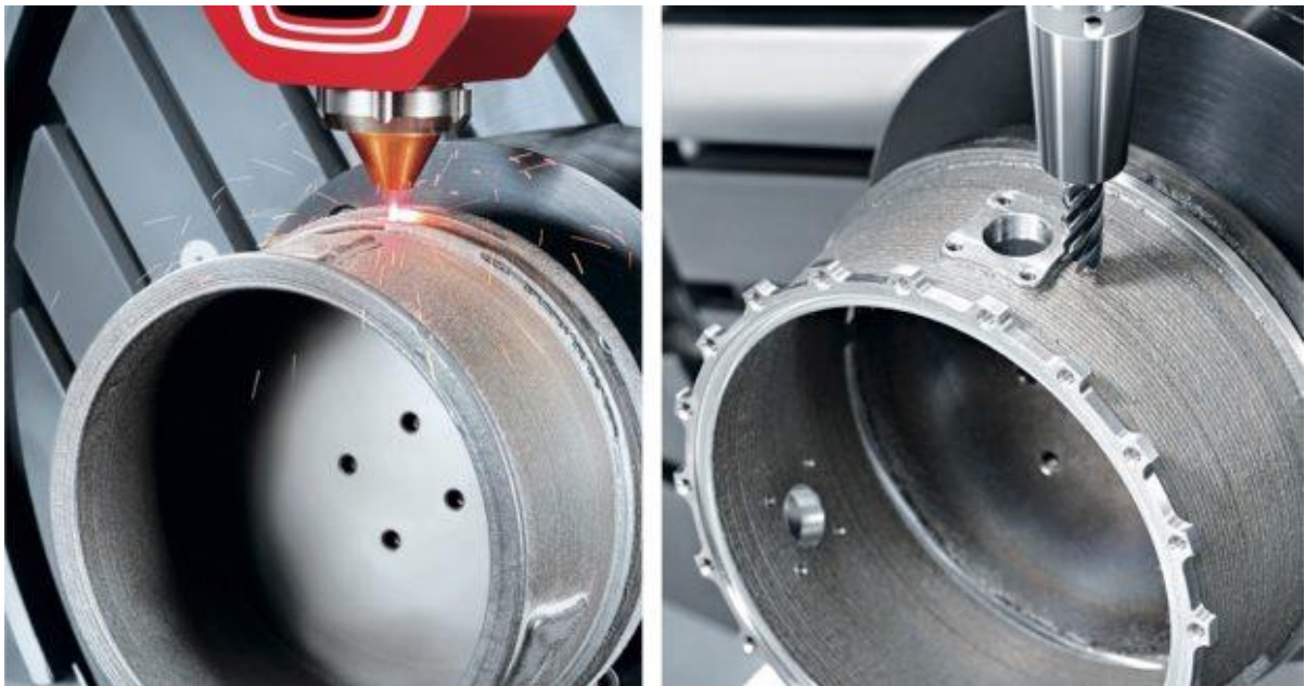
Figure 2-4 DED hybrid process (DMGMORI 2017)
